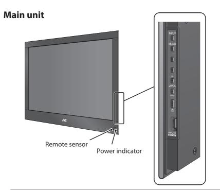
Power indicatorLights while the monitor is on.Remote sensorAim the remote control here.
